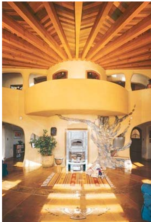
Living room Rastra walls, recycled timber ceiling.
